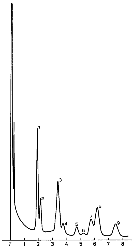
Fig. 1. Gas chromatogram of partly methylated alditol acetates derived from B and C : 1, 2,3,6-tri- O -methylmannitol triacetate; 2, 2,3,6-tri- O -methylglucitol triacetate; 3, 2,3-di- O -methylmannitol tetraacetate; 4, 2,3-di- O -methylglucitol tetraacetate; 5, 2- O -methylmannitol pentaacetate; 6, 2- O -methylglucitol pentaacetate; 7, 3- O -methylmannitol pentaacetate; 8, mannitol hexaacetate + 3- O -methylglucitol pentaacetate(?); 9, glucitol hexaacetate. T values relative to that of 2,3,4,6-tetra- O -methylglucitol diacetate.
